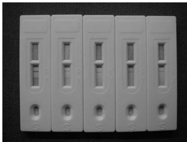
Figure 4. Strip test for the detection of MEL in animal feed (concentrate feed). The spiked levels used were 0, 1.0, 1.5, 2.0, and 2.5 \mu\text{g/g} from left to right. The level of 2.0 \mu\text{g/g} MEL in animal feed causes complete disappearance of the test line.
