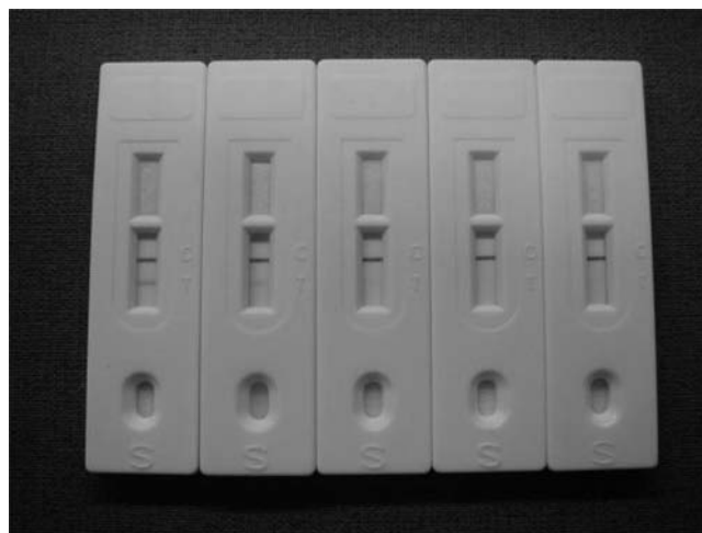
Figure 5. Strip test for the detection of MEL in milk powder. The spiked levels used were 0, 0.5, 0.8, 1.0, and 1.2 \mu\text{g/g} from left to right. The level of 1.0 \mu\text{g/g} MEL in milk powder causes complete disappearance of the test line.
