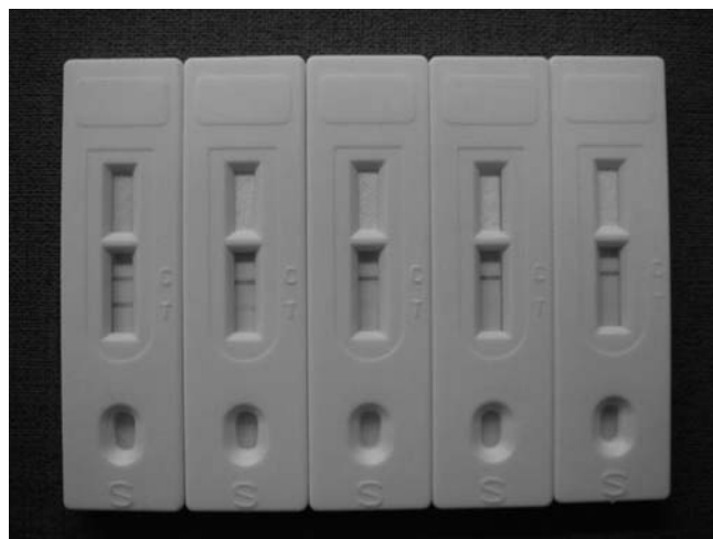
Figure 3. Strip test for the detection of MEL in raw milk. The spiked levels used were 0, 0.01, 0.03, 0.05, and 0.1 \mu\text{g/mL} from left to right. The level of 0.05 \mu\text{g/mL} MEL in raw milk causes complete disappearance of the test line.
